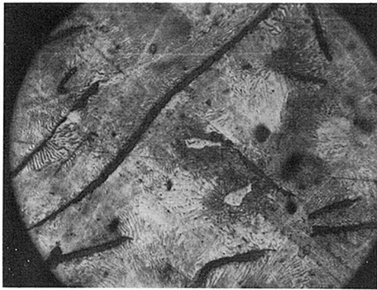
Fig. 1(a) Microstructure of gray iron, 550x
