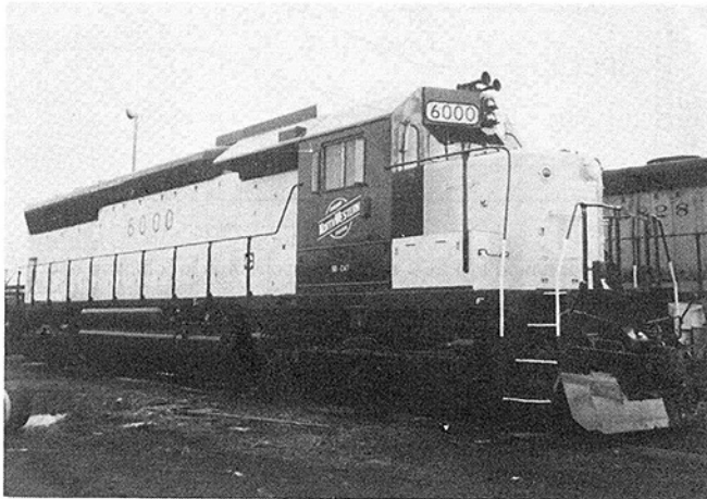
Fig. 9 Chicago-Northwestern 3612 repower of an EMD SD45 locomotive
