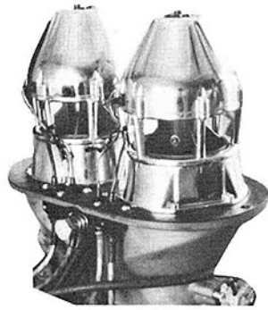
Fig. 7 Specially instrumented carburetor
