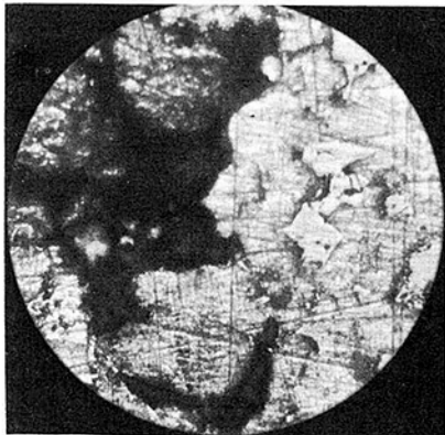
Fig. 7(a) Unworn 390Al specimen, 175x
